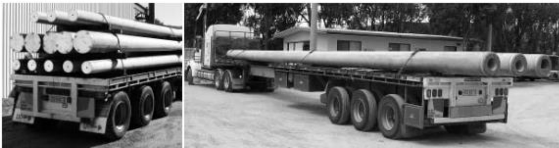
Length of the Vehicle Bed for Transportation of Pre-stressed Concrete Pole
